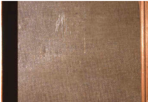
Figure 25.5 Detail of the reverse of a painting wax lined in 1965, in raking light (Mauritshuis inv. no. 166). Excess wax-resin adhesive is visible. Photograph by the author
