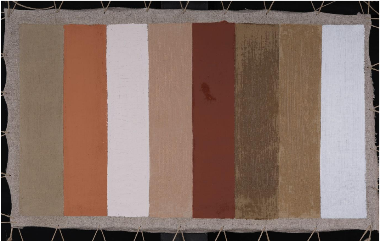
Reconstruction #B5 before wax-resin impregnation (22 July 2024)
